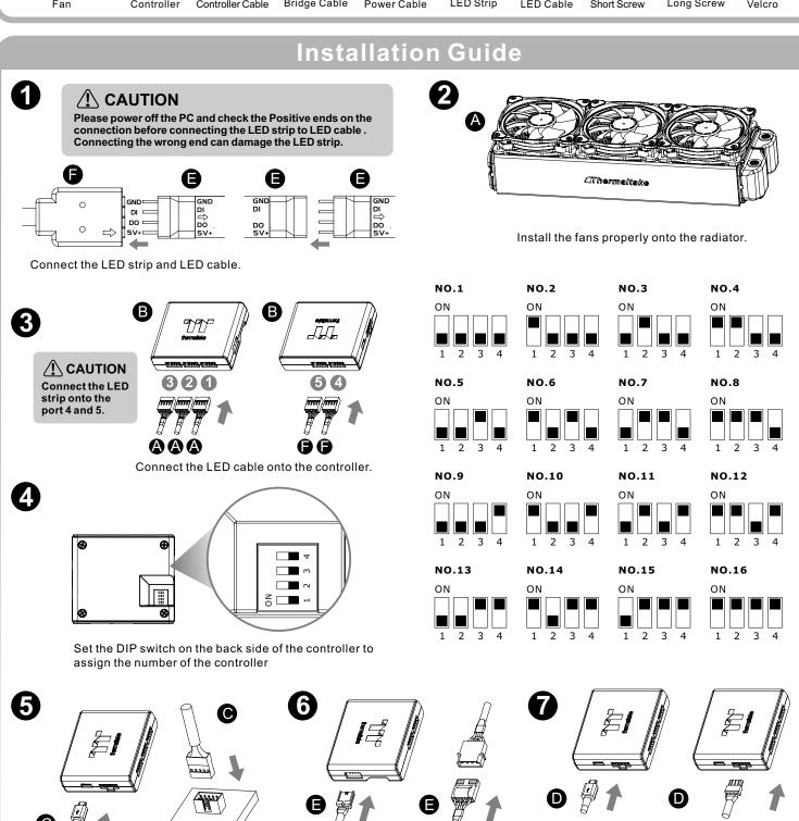
Connect the controller cable onto the mainboard (USB 2.0 9 pin) and controller.
